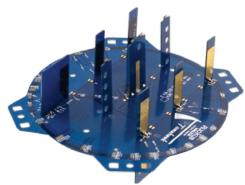
Dual-polarized (horizontal and vertical) antenna elements increase reliability through antenna diversity and optimize performance for a wide range of client devices
