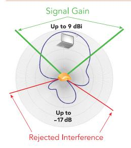
BeamFlex not only focuses RF energy only where its needed but also nullifies interference coming from other directions. This ensures that the highest possible PHY rate is used and that the highest possible throughput is achieved for all clients.
